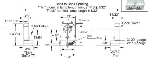
Wire Fast Terminals Individual Wire Holes (2 per contact)
